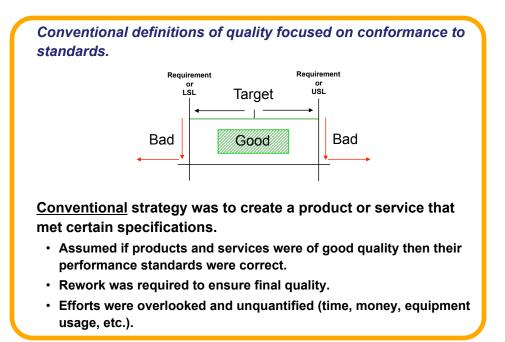
Using this strategy often required rework to ensure final quality or the rejection and trashing of some products and the cost of the efforts to accomplish this "inspect in quality" were largely overlooked and un-quantified.
