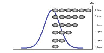
The likelihood of a defect decreases as the number of Standard Deviations that can be fit between the Mean and the nearest spec limit increases.
