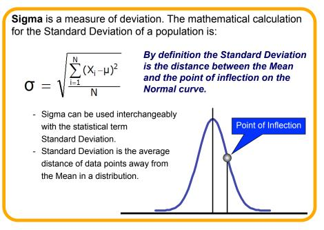
When measuring the sigma value of a process we want to obtain the distance from the Mean to the closest specification limit in order to determine how many Standard Deviations we are from the Mean...our Sigma Level! The Mean being our optimal or desired level of performance.
