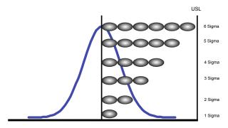
The likelihood of a defect decreases as the number of Standard Deviations that can be fit between the Mean and the nearest spec limit increases.
