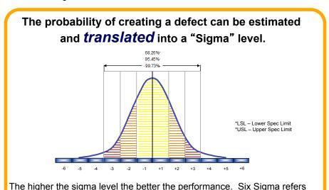
to a process having 6 Standard Deviations between the average of the process center and the closest specification limit or service level.
