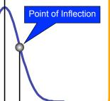
When measuring the sigma value of a process we want to obtain the distance from the Mean to the closest specification limit in order to determine how many Standard Deviations we are from the Mean....our Sigma Level! The Mean being our optimal or desired level of performance.
